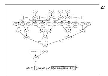
The Boolean circuit for the truth function the reduction uses for this particular input. The circuit for " $x \in [[e]]^L$ " depends on e and x, but not on L.
